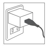
Insert the USB plug of DC cord into the AC adaptor provided and then plug AC adaptor into a power outlet.
